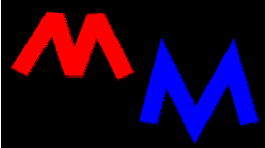
The red M has a miter limit of 0 - notice the chopped off corners. The blue M has a miter limit of 4 so the corners are fully formed.
