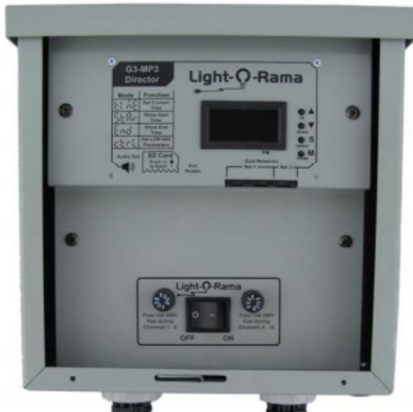
G3 MP3 Director as part of an LOR1602MP3g3. LOR1600MP3g3 similar. Note: the LOR160xg3 looks similar but does NOT have an MP3 Director
