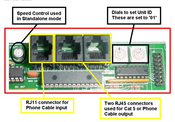
Once AC power has been supplied to the CTB08D the **red LED** will begin to blink. This is an indication that the Unit is functioning and that there is NO COMMUNICATION. Once communications is established, the LED will stop blinking and it will light steadily.
