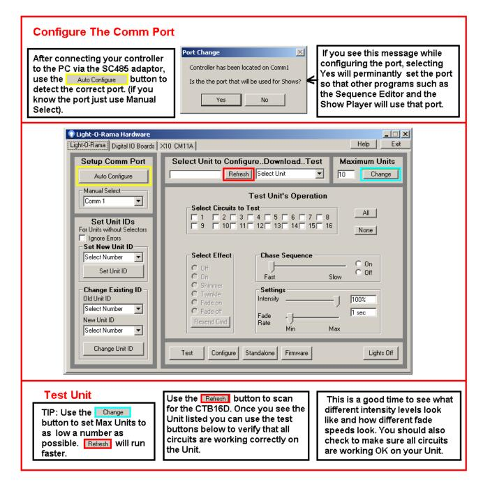
**IMPORTANT:** When developing a Sequence to control the lights, the sequence must refer to the CTB08D's Unit ID or the lights will not blink. This is true if the sequenced is going to be downloaded as a **standalone** sequence as well as if the CTB08D is controlled via the PC.
