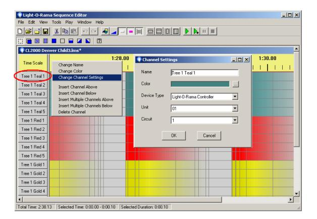
In the Sequence Editor, click on a channel box (on the left of the screen). In the menu that pops up, select *Change Channel Options*. You can then Set the Device type to Light-O-Rama Controller and the Unit to the ID that you picked for this Unit. You will also notice that you can specify a Circuit Number. Circuit number 1 corresponds to Output Circuit 1 on the board.
