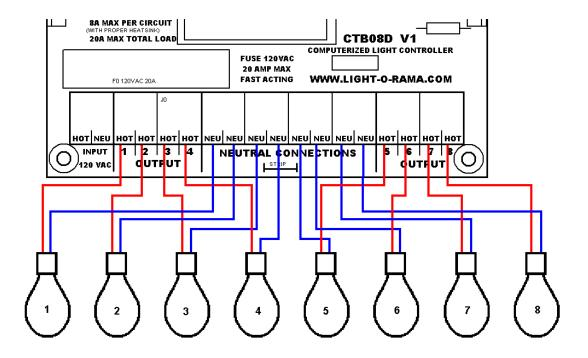
Note: Neutral wires can be placed in any of the 8 neutral connections on this card. Order of placement is not important.
