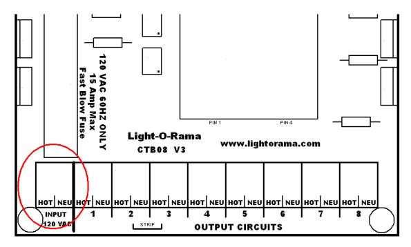
Power coming into the CTB08 is connect on the terminal circled in red. Two wires are connected, a HOT and a NEUtral. Power must be 120 volts AC 60HZ.
