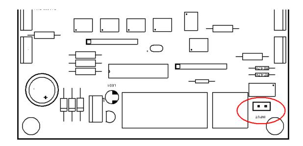
The input connector noted above is used during standalone operation of the unit. When used in standalone mode, the CTB08 can operate without a connection to the PC. To operate in this mode, an animation sequence must be installed on the CTB08 using the Light-O-Rama Hardware Utility. See the HELP files with the Hardware Utility for sequence download instructions.
