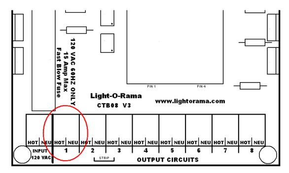
Each output circuit of the CTB08 can handle 2amps without a heat sink. 8 amps with proper heat sinking. There are 8 output channels with HOT/NEU connections. Neutrals can be connected off the card if that is more convenient.
